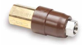
Parker's vent line breakaway provides an important safety feature for CNG dispensing systems. It allows the vent line hose to safely disconnect, preventing damage to the dispenser in the event of a "drive off" and allows any CNG remaining in the vent line to bleed off safely.
